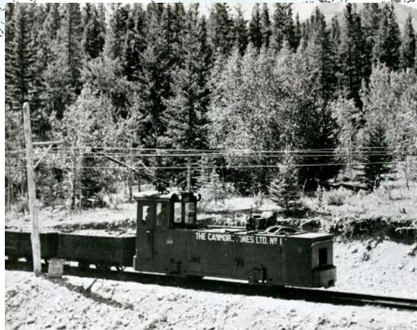
Canmore Mines Ltd. narrow gauge electric locomotive hauling coal from the No. 3 Mine to the tipple at the No. 2 Mine. CMAGS 1983.001.127.001
